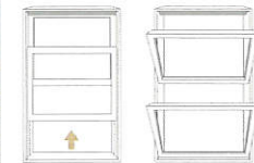
Single Hung Double Hung Single Hung: Min 1'6"x2'0" Max 4'0"x7'0" Double Hung: Min 1'6"x2'6" Max 4'0"x7'0"
